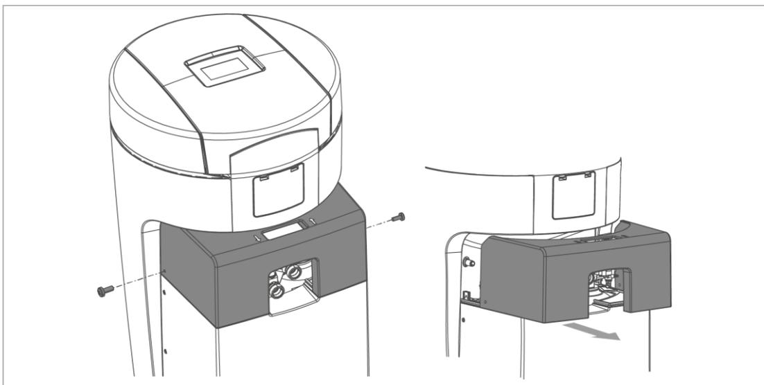
1. Loosen both screws on the side of the upper part of the housing for the technical equipment.
